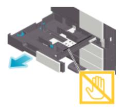
• When loading envelopes of which the length is 7-3/16 inches (182 mm) or less, mount the Attachment on the Lateral Guide.
