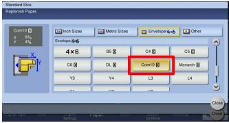
\*NOTE: Large and odd size envelopes can also be run in Tray 1 and would need to be set up as "Custom Size". They can also be done in the BYPASS TRAY (\*maximum 10 envelopes in Bypass Tray).
